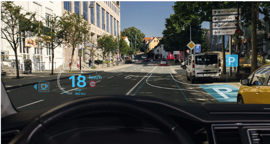
Holographic augmented reality head-up displays based on ZEISS „Multifunctional Smart Glass“ technology project important information without drivers having to take their eyes off the road. Photo: © ZEISS
